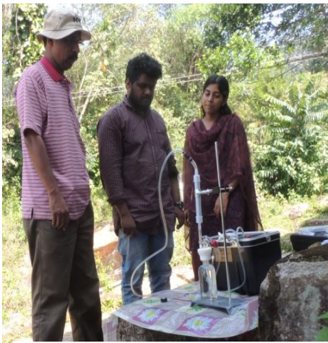
Onsite measurement of radon concentration using RAD7
